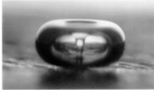
Figure 4. Crum's photograph of jet formation during bubble collapse
